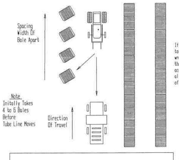
If bales are brought to the site before wrapping, arrange then to allow easy access to hales and allow tubeline plenty of roan to nove
