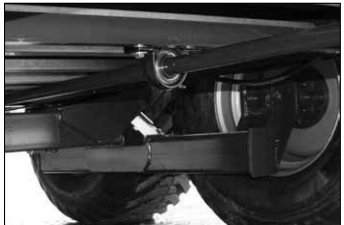
Grease 3 fittings on PTO driveline underneath spreader at front, middle, or rear crossbars.
