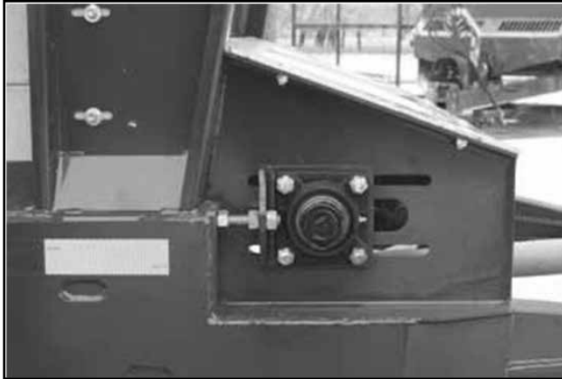
Apron chain bearing grease zerk, located at front and rear of spreader on both sides.
