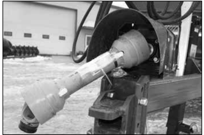
Grease all fittings on the PTO driveline.
