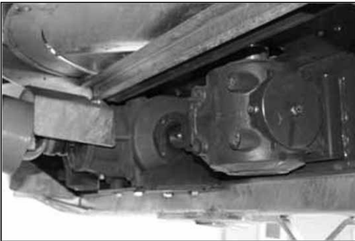
Check oil levels in gearboxes, top up with SAE 80W90 gear oil if needed.
