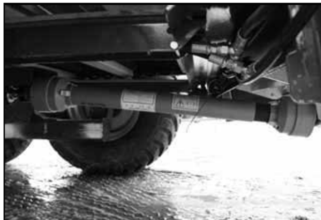
Grease all fittings on rear PTO shaft.
