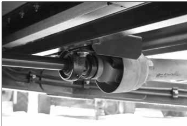
Grease zerk on PTO drive line bearing.
