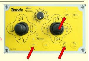
Adjust actual bed speed to 'just stopped' using "Raise Knives" button to lower speed or "Lower Knives" button to raise speed.
