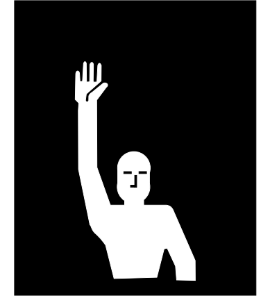
Fig. 5 STOP. Raise arm straight up, palm to the front.
