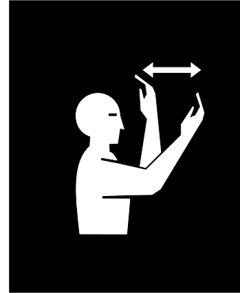
Fig. 3 MOVE TOWARD ME FOLLOW ME. Look toward person or vehicle you want moved. Hold one hand in front of you, palm facing you, and move your forearm back and forth.
