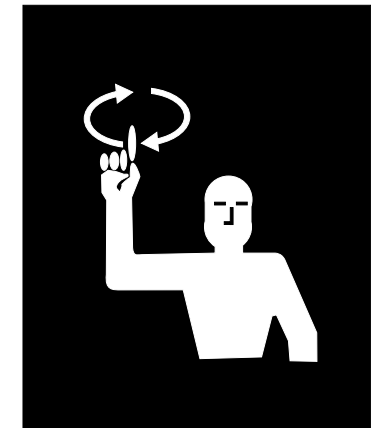
Fig. 11 RAISE EQUIPMENT. Point upward with forefinger, while making a circle at head level with your hand.
