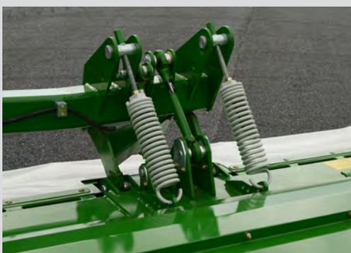
Most rear mowers have a central pin which allows the mower to move left and right to adjust to changes in ground condition. The McHale Pro Glide is different in that it is fitted with a patented 3D ground tracking suspension unit, which allows the mower to:
