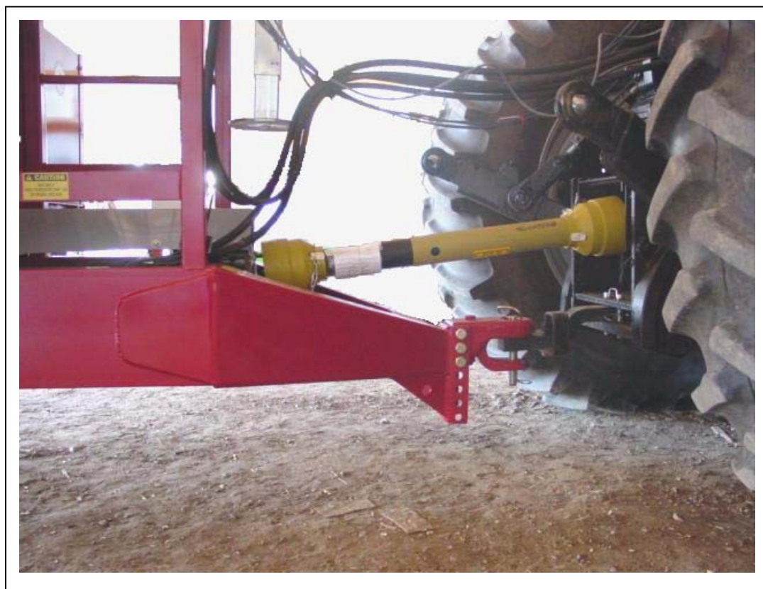
Figure 9 - Typical Attachment to Tractor showing Hitch hookup, PTO shaft hookup, Wire harness and Hydraulic Connections.
