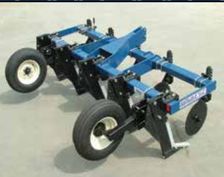
Optional StripTill mounting attaches to ShearBolt shanks
